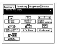
5 Touch [X] or [Y], and use the keypad to enter the desired zoom ratio, and then touch [Enter].
