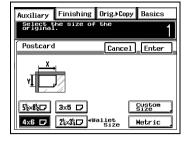
○ For a paper size other than the standard sizes listed on the screen, touch [Custom Size]. Touch [X++], [Y++], [▼], and to specify the the size of the original, and then touch [Enter].
